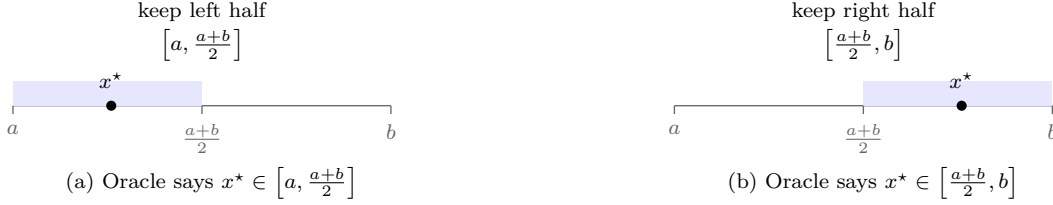
Figure 1: In one dimension, querying the center of mass means querying the midpoint. The separation rule returns one of two half-intervals, and the localization length is cut exactly in half.
